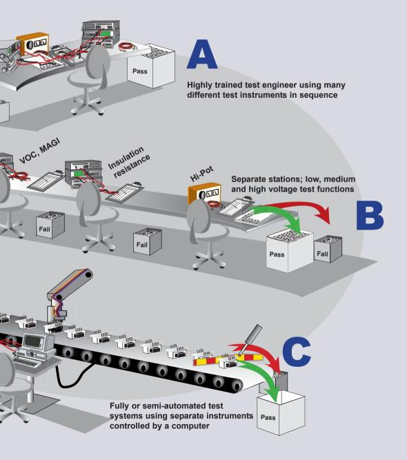
For many years, test instrumentation available to the transformer market has limited manufacturers to one of these testing methods. Unfortunately, these methods may have a number of problems:
