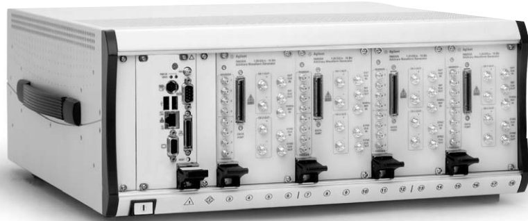
Figure 4. Four N6030A modules fit conveniently inside an 18 slot CompactPCI chassis.
