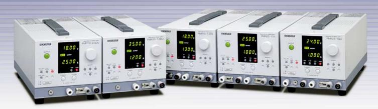
The PMR Series is a multi-output, constant voltage/constant current regulated DC power supply with a dual-tracking function. It uses a series regulator system to generate stable outputs with low noise. Moreover, it is compatible with various external controls.
