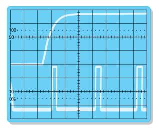
The high slew rate of 0.7V/µs and the minimum pulse width of 100µs in the arbitrary mode allow simulation of complex dynamic load conditions. Using external modulation, almost any waveform can be obtained in the frequency range up to 8kHz. This allows the HM8142 to be used as a
