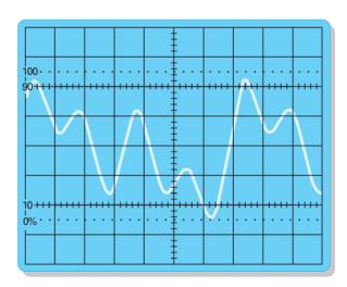
power amplifier or high power function generator. The linear output stage ensures low distortion over the entire operating range. Arbitrary waveforms can easily be designed by simply entering voltage and time parameters by means of the IEEE-488 or RS-232 interfaces.
