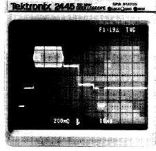
This sample waveform and CRT readout show a 2445's high-fidelity display of the Vertical Interval Reference Signal on Line 19, Field 1 with the television blanking-level clamp (TVC) engaged. The instrument used is also equipped with Option 10 (GPIB).
