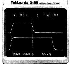
Your eyes never have to leave the screen to obtain front panel settings and measurement results. In the CRT example above, the top area of the display
