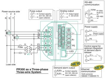
Other RS-485 devices can be connected to the network using Ethernet-serial gateway function
