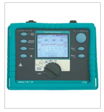
The measured parameters are sampled at 10.24kHz, can be recorded over time and displayed on the colour screen in chart mode and downloaded to a PC for further analysis and report generation. The chart mode facility is ideal for identifying intermittent problems, trends with time and peak demand figures. The firmware of **ANALYST 3P** can be updated via a standard RS232 interface.
