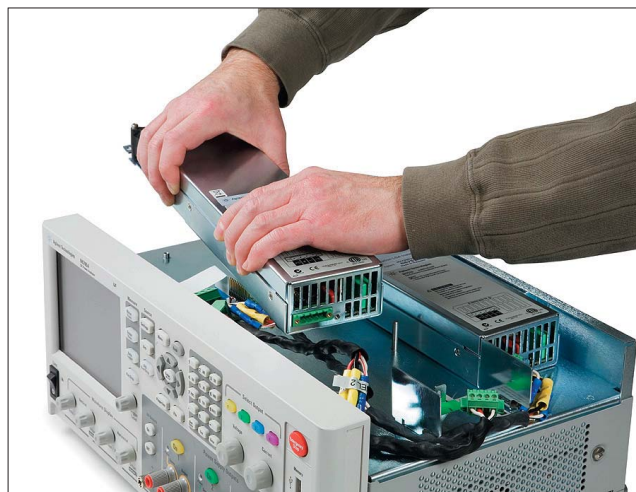
Figure 2. DC Power Modules are easily installed into the N6705A DC Power Analyzer Mainframe.
