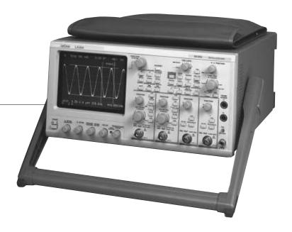
With four channels and 500 MHz bandwidth, these leading-edge oscilloscopes offer the highest level of analog performance available today.
