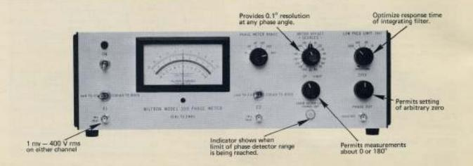
This general purpose phase meter makes accurate phase measurements from 10 Hz - 2 MHz with 1 mv sensitivity, and provides high input impedance and wide measurement capability.
