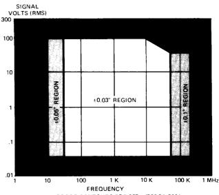
TYPICAL ERROR CONTOURS FOR 305 w/305-PA-3001 FOR UNEQUAL INPUTS - REF. 0.3 VOLTS RMS
