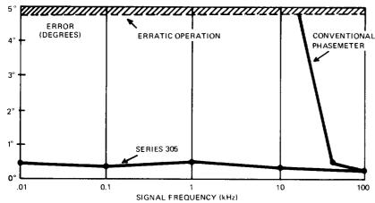
PHASE READING ERROR VS SIGNAL FREO. FOR GAUSSIAN NOISE (FLAT TO 5 MHz) IN BOTH CHANNELS FOR S/N = 10
