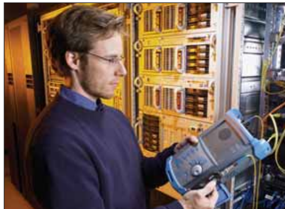
EXFO's premises network OTDR configurations offer the shortest dead zones in the industry, controlled launch conditions and, ultimately, pinpoint accuracy for loss measurements.
