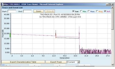
OTDR Trace Viewer displaying a fault along with reference
