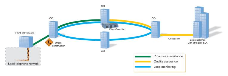
Typical configuration of a Fiber Guardian test application
