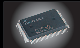
Specially-designed gate array with built-in CPU
