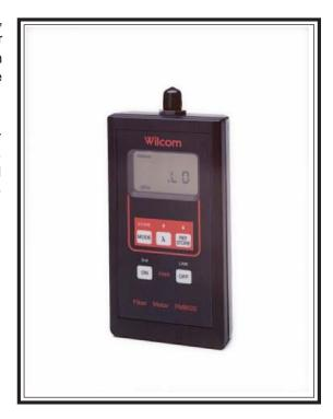
Model FM1317 measures power from +5 dBm to -70 dBm with calibrated wavelengths of 850, 980, 1310, 1480, 1550 and 1625nm making this unit ideal for singlemode, multimode and WDM fiber optic testing. Additionally, 2 kHz signal detection is performed by the unit for easy fiber identification.
