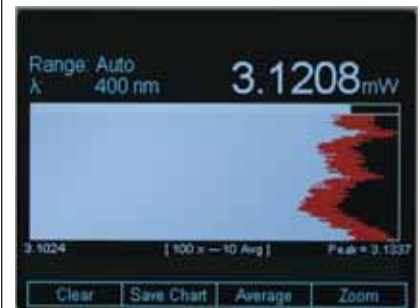
The 1918-C with vertical strip chart display
