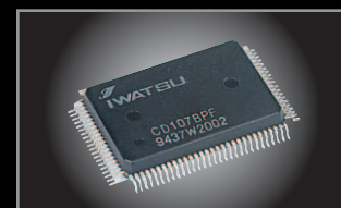
Specially-designed gate array with built-in CPU
