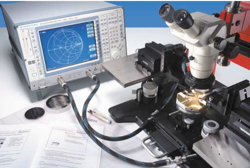
The Rohde & Schwarz calibration techniques offer maximum convenience and accuracy also for on-wafer measurements
