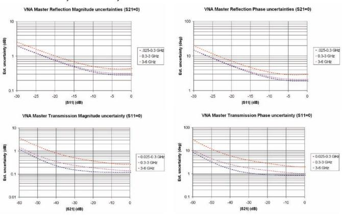
The uncertainty graphs above provide measurement uncertainty at 23° C after vector correction for the standard N connector type. Errors are worse-case contributions of residual directivity, source match, frequency response, network analyzer dynamic range, and connector repeatability. For the 1-path 2-port measurements, transmission tracking, crosstalk and physical load match termination was added. OSLN50-1 calibration components were used.
