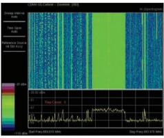
With Option 25, spectrogram measurements identifies intermittent interference.
