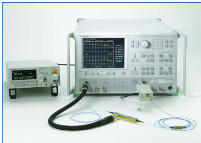
E/O measurement of an optical modulator
