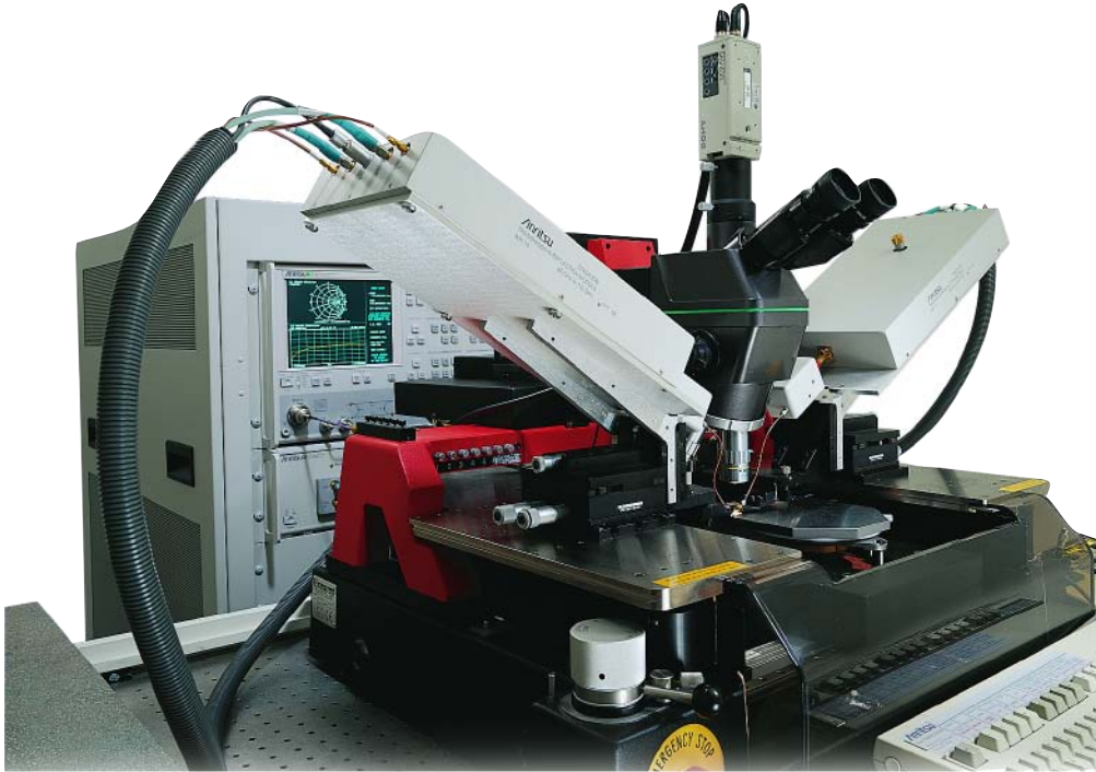
On-wafer measurements to 110 GHz with the ME7808B
