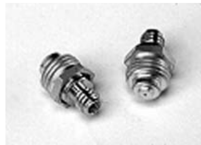
Figure 11. A pair of 1.0 mm female connector launch assemblies. Left: 1.0 mm female connector end. Right: package end with 0.162 mm diameter pin.
