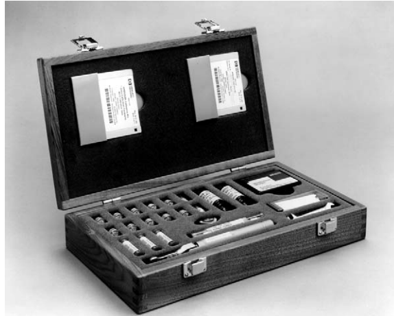
Figure 9. Agilent 85059A, 1.0 mm calibration/verification kit
