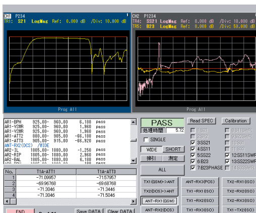
Example of pass/fail evaluation of a multi-port device used for communication
