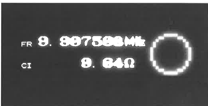
▲ GO/NO-GO testing of a crystal oscillator
