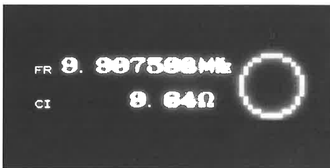
▲ GO/NO-GO testing of a crystal oscillator
