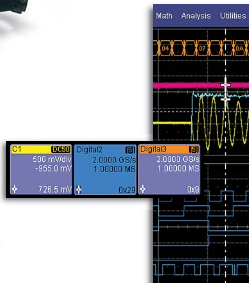
Use oscilloscope tools like horizontal and vertical cursors along with automatic measurements and statistics to measure analog and digital signals.
