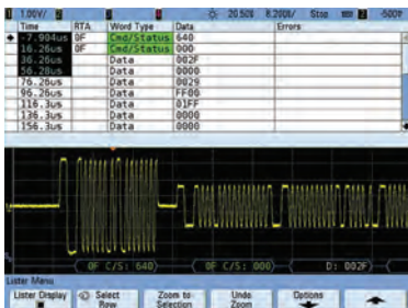
Time-correlated display of the MIL-STD 1553 physical layer signal with protocol decoding.
