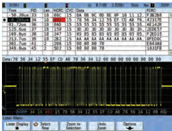
Time-correlated display of the FlexRay physical layer signal with protocol decoding.
