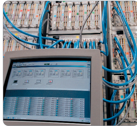
► Up to 8,160 logic analyzer channels acquire real-time data.
