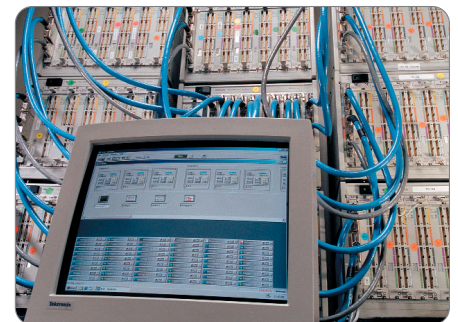
► Example of TLA721 with ten TLA7XM Mainframes.
