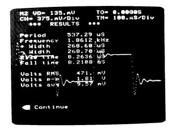
HP 19860A waveform characterization—the HP 19860A Digital Waveform Storage option and the HP Waveform Measurement Library can automatically characterize waveform parameters. This photo shows measurement results from the first-day Automatic Waveform Measurement Program. The program accounts for the ringing on the waveform when measuring parameters such as rise time and fall time. This program provides first-day measurement results without requiring any additional programming.
