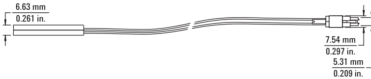
Figure 3.6. E5394A and E5396A soft touch probe dimensions
