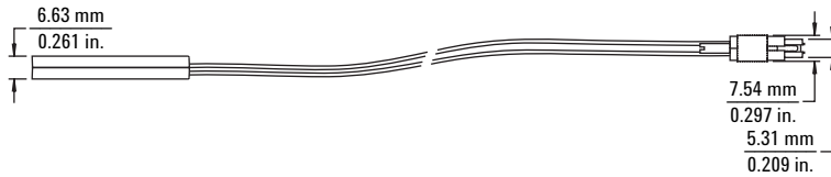
Figure 3.6. E5394A and E5396A soft touch probe dimensions
