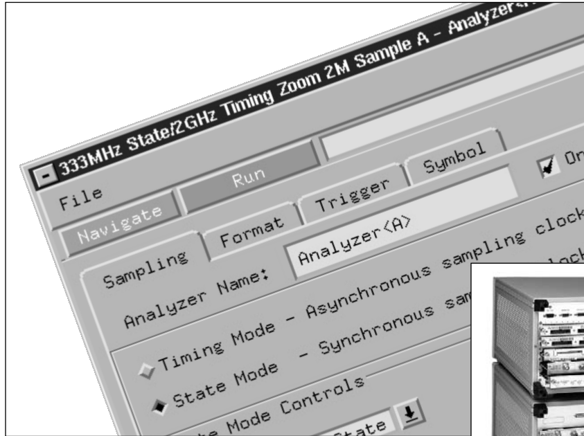
Figure 2. Acquire state data at 333 MHz and timing data at up to 2 GHz through the same connection.
