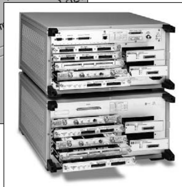
Figure 3. Configure your HP 16700A Series system for your specific application with modular mainframes.
