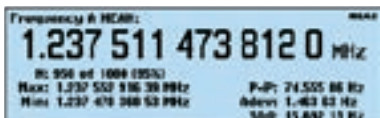
Figure 6: The Numerical Statistics mode shows different statistical parameters at the same time.
