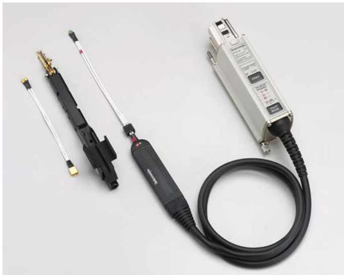
P7500 TriMode probes simplify complex measurement setups.
