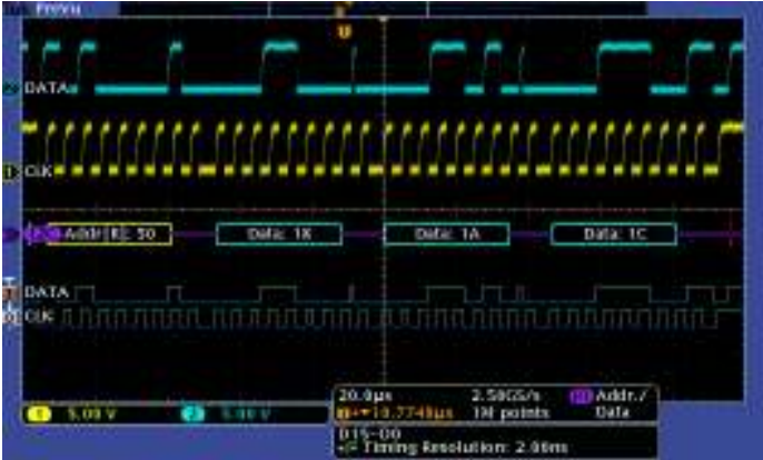
Triggering on a specific data packet going across an I 2 C bus. The yellow waveform is clock and the blue waveform is data. A bus waveform provides decoded packet content including Start, Address, Read/Write, Data, and Stop.
