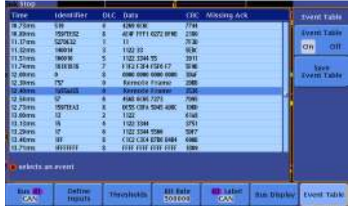
Event table showing decoded Identifier, DLC, DATA, and CRC for every CAN packet in a long acquisition.
