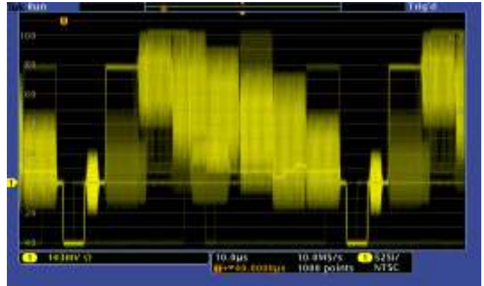
Viewing an NTSC video signal. Notice the intensity-graded view provided by the DPO's ability to represent time, amplitude, and distribution of amplitude over time.
