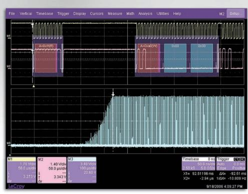
allows triggering on a range of DATA bytes that correspond to reads or writes to specific sub-address memory blocks in the EEPROM. It can also aid in monitoring DATA outputs from I<sup>2</sup>C-based sensors, such as analog-to-digital converters, and triggering when DATA is outside a safe operating range. In both cases, verifying proper operation becomes a simple task.
