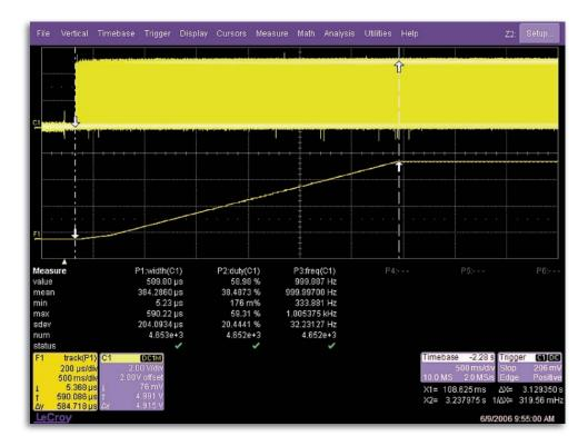
The PWM signal for a power tool motor speed controller is monitored during start-up. The Width parameter is used. All instances of Width during the acquisition are measured. Then, Track was applied to determine when the speed plateaued (i.e., when the tool rotation reached steady-state).
