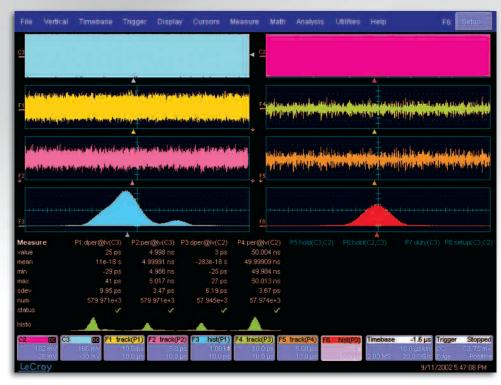
A 200 MHz clock signal is acquired at 10 GS/s using 20 Mpts of acquisition data (400,000 cycles). Cycle-Cycle and Period Jitter are measured and analyzed with Tracks and Histograms. Cycle-Cycle jitter shows a distinctive modality. Other signals could now be acquired and time-correlated to understand the histogram modality.
