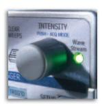
WaveStream is most helpful in viewing signals that have signal jitter or signal anomalies, or
