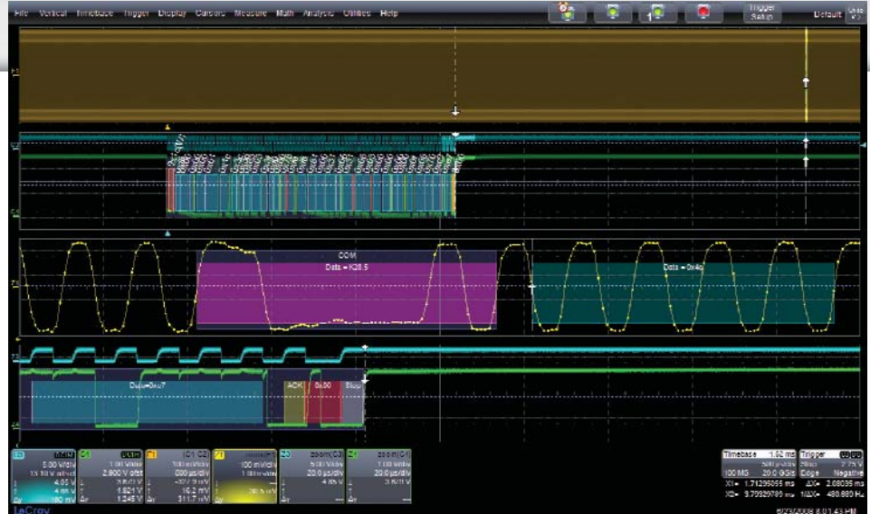
Capture 5 ms (100 Mpts) of low-speed and high-speed waveforms. Easily zoom, and validate timing relationships between signals.
