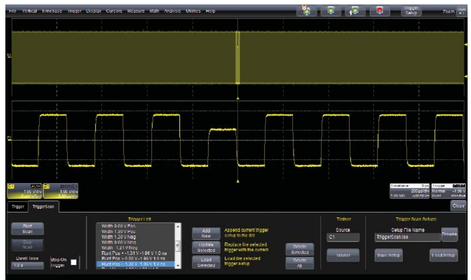
A 1 in a billion rare event seems fast but is only 5 seconds of circuit operation on a 200 MHz clock. TriggerScan finds the rare event in 4 minutes while an oscilloscope with 400,000 waveforms/second capture rate misses 99.8% of the signals and could spend nearly 42 minutes to find the error.
